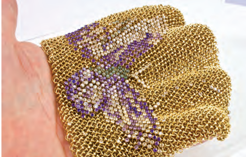
The greatest potential for additive manufacturing technology is in complex designs that are difficult or impossible to produce by casting. The mesh bracelet shown here, which was designed by Digital Forming for Cookson Precious Metals, is one example.
